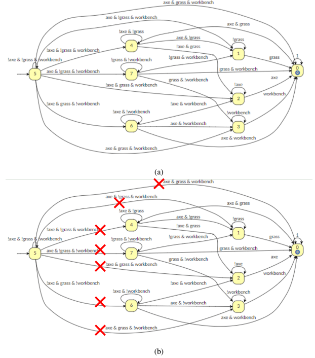
Figure 9: Figure 9a depicts the reward machine for the the specification \varphi_{\text{test}} = \mathbf{F}_{\text{workbench}} \wedge \mathbf{F}_{\text{grass}} \wedge \mathbf{F}_{\text{axe}} as well as all feasible edges matched by the Relaxed criterion. Note that all the edges have at least one matched transition-centric option for the Relaxed criterion. Figure 9b depicts the edges that do not have a compatible transition-centric option for the Constrained edge matching criterion.
