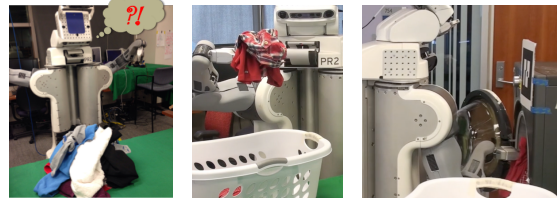
Figure 1: PR2 robot doing the laundry using our planning approach for addressing partial observability and non-determinism.
