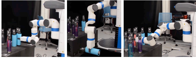
(a) The Fetch mobile manipulator uses a STAMP policy to pickup a target bottle while avoiding those that are likely to be crushed. It replaces a bottle that wasn't crushed (left), discards a bottle that was crushed (center) and picks up the target bottle (right).
