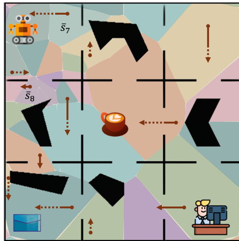
Figure 1: In a continuous version of the office domain, the agent needs to learn policies for delivering multiple items. Polygonal cells illustrate learned state abstractions, and arrows illustrate learned policies with abstract actions parameterized by parameter intervals. Each arrow corresponds to an interval [a, b] of possible movement values: the solid segment indicates the lower bound a , and the dotted segment indicates the interval width b - a . Narrower dotted segments denote higher precision in the learned action parameters.
