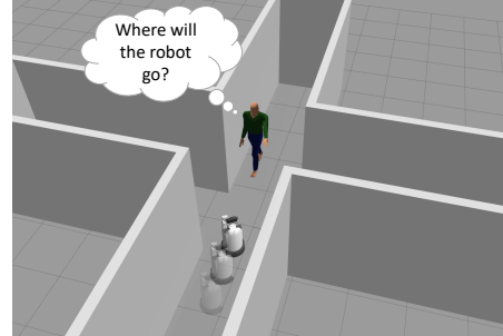
Fig. 1: An example of a social navigation scenario in a confined environment where the robot’s movement can not reveal any information about its future intentions.
